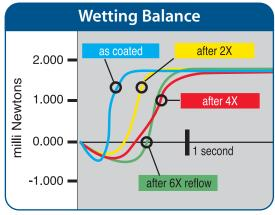
The wetting balance curves above clearly illustrate M-Coat's durability, quick wetting characteristics, and consistently strong protection of copper.
