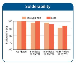
The M-Coat process produces a durable finish that solders effectively after multiple heat excursions. Its compatibility with a broad range of fluxes assures a simple and trouble-free assembly.
