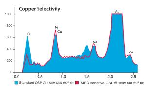
M-Coat Select is formulated to coat copper surfaces selectively, leaving no residue or unsightly film on gold surfaces. The spectra above clearly highlights how a conventional OSP process leaves organic materials on the gold surface (blue trace.) M-Coat Select coats only the copper leaving no contamination on the gold surface (red trace.)
